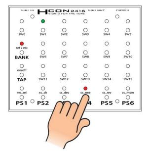
Press sw3 to change the value of the single digit to 3. Then cc\_one LED will blink. To check the previous value, press cc\_one.
