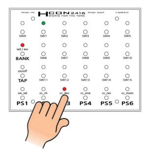
Press sw12 to change the tenth digit to 120. Then, cc\_dec LED will start blinking. To check the previous value, press cc\_dec.
