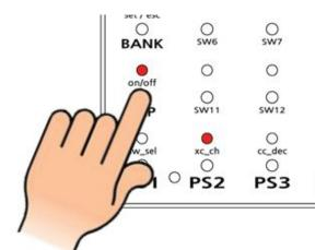
Pressing the Tap switch will result in both loading the default template and clearing all of the saved presets.
